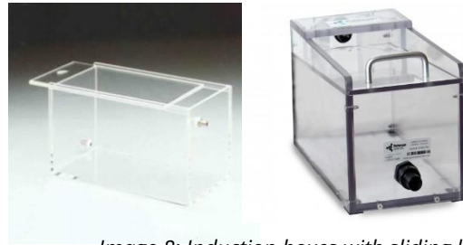
Image 8: Induction boxes with sliding lid
